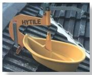
wheel widens. Don't just slide the chisel down and nip up the grubscrew – it will pop back up with the first cut. Instead, pack some small washers under the base of the chisel. Replace the wheel from time to time and also the small pin that goes through the wheel. Worn bolts in the handle and plunger linkage can be replaced with our special oversize bolts. If you prefer, we will do the maintenance for you while you wait.
