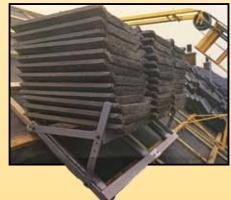
The Hytile Batten Trolley is a popular tool for the "back conscious" roof tiler. Tiles can be transferred from one end of the roof to the other with a minimum of physical effort.
