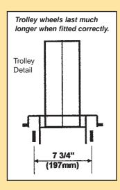
**Trolley Wheels** – When fitting new trolley wheels, ensure them of a long life by following these three simple steps:
